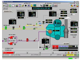
Boiler efficiency can have a big impact on plant fuel gas costs. High levels of oxygen in the stack gases indicates that the boiler is operating at suboptimal efficiency. This is typically due to:
