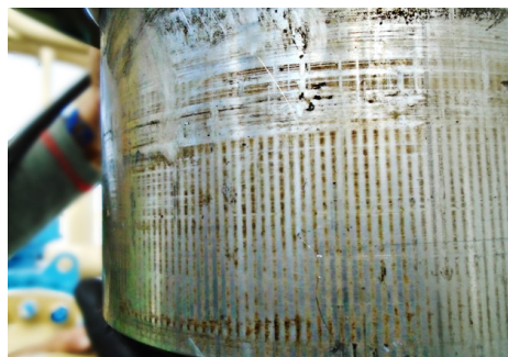
Weld slag found in a valve after flushing lines damaged the valve trim. Cost for new trim was $30,000 with a 13-week lead time.
