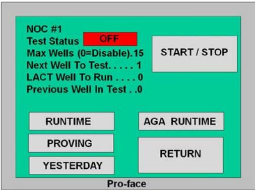
**Runtime:** The **Runtime** screen allows the user to see all the process variables while a well is in test. Touch the **Return** button to go back a screen then touch the **Proving Screen** button.
