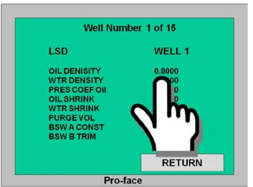
Make the change required to we the oil, water or gas variable then touch ENT to accept the change.
