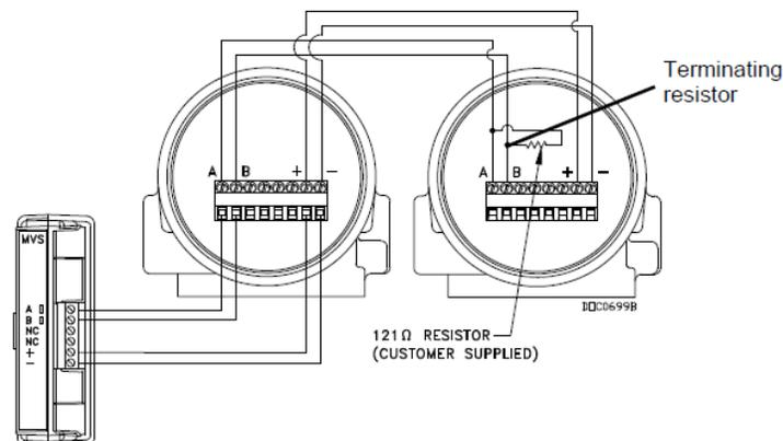
*Figure 6-2* shows a terminating resistor—typically a 121  $\Omega$  customer-supplied resistor—on the last transmitter in the multi-drop. This resistor correctly terminates the multi-drop configuration.
