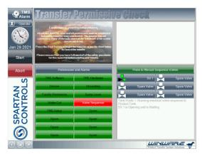
\* During a transfer, any required alarm condition, including high tank and water cut levels, can be configured to alert the driver with a beacon or horn actuation. TMS records unauthorized transfers and can alert your operations personnel.
