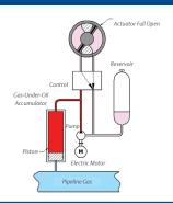
In the first sequence the actuator is in the open position awaiting a demand to close signal. The valve may be operated locally, remotely or automatically by a variety of sensory and control devices. Until a demand signal is received, the piston accumulator remains in the fully charged state at the same pressure as the pipeline.
