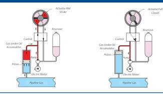
In the second sequence, the actuator has received a demand to close signal and the actuator control system opens the flow paths to the rotary vane. The pressurized gas in the accumulator forces hydraulic fluid into the actuators closing port and powers the actuator in the clockwise direction. At the same time, non-pressurized fluid from the actuator's opening port returns to the reservoir. Finally, the actuator has reached the fully closed position.
