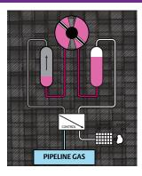
Eliminate high pressure vented emissions Using pipeline gas to pressurize hydraulic fluid and actuate the valve, the ECAT eliminates high-pressure gas venting from the tanks through the control panel.
